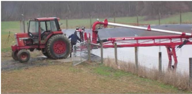
During any manure movement or mixing, operator must be up above the ground and away from edge of a manure storage. Particularly with manure containing gypsum bedding material,  $H_2S$  gas at lethal levels (>600 ppm) is quickly produced and undetectable by smell. Hydrogen sulfide is a heavy, ground-hugging gas.
